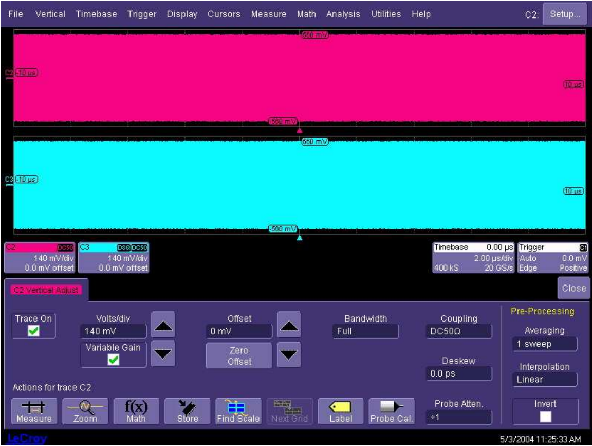
Figure 13. Signals properly adjusted for best accuracy
